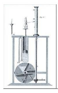
In Ctesibius's clepsydra from the 3rd century BC, the humanshaped hour pointer ascends as water flows in. Outflow drives a series of gears that rotate a cylinder bearing hour lengths appropriate for each day's date.
